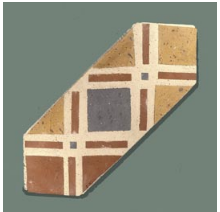
The individual 'masonry tiles' had a rebate all around them, which formed a network of 50 mm (2") grooves all over the face of the giant column. A mirror-polished stainless steel flat was bolted into the groove. This one 'tile' was the only piece of 'mock-up' which Rosehaugh-Stanhope would fund. JOA paid for the remainder ourselves - subsequently aided by the Biennale 1991 budget! Not very 'American' at all!
